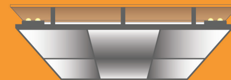
Drop ceiling with perimeter lights
