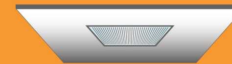
LED lights recessed in canopy
