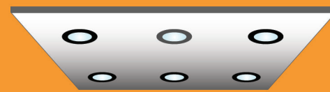
LED downlights recessed in canopy
