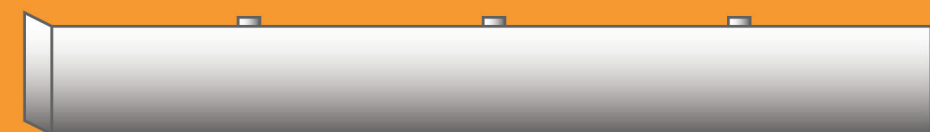
Bumper rails (SS #4 Flat Bar 6" x 1/4")
