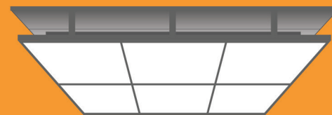
LED lights with lexan diffusers in drop ceiling*
